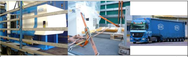
Machines are loaded unpacked (incl. dust protection cover) by crane from above on the truck. If loaded on an open loading platform due to oversize, a tarpaulin is needed to cover the machine completely!
