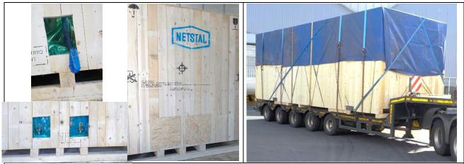
Packaging is only "brought along" – load securing points are on the machine. / Important: be absolutely sure to close the baffles on the crate!
