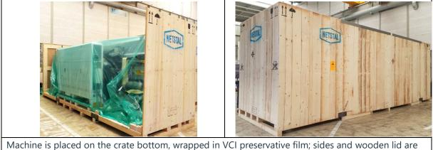
Machine is placed on the crate bottom, wrapped in VCI preservative film; sides and wooden lid are connected to each other.
