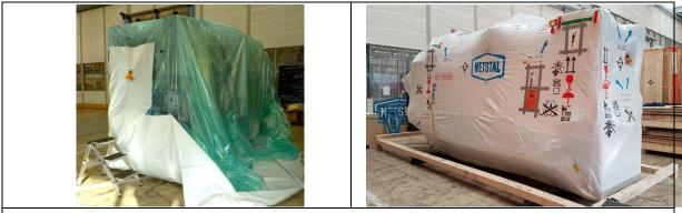
Machine is placed on steel-reinforced wooden bottom including fender, is wrapped in VCI preservative film and additionally will be shrink-wrapped in polyethylene film.
