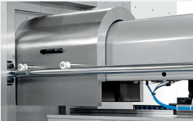
Actively controlled shut-off nozzle actuation
